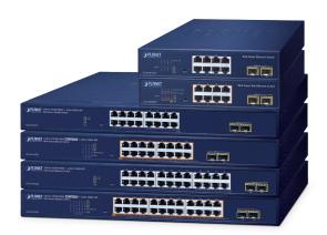
**PLANET GS-2210 smart Ethernet switch** combined with **NMS** makes network management easier and more efficient. In addition, it is easy to configure whatever application that the industry needs. It features link aggregation, IGMP, QoS, PoE schedule and more to improve the availability of critical business applications.
